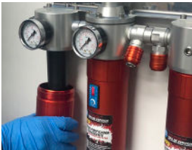
Unscrew lower section
