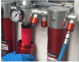
Unscrew lower section
